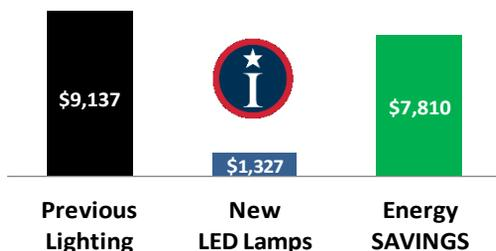
**Results** Reducing the fixture wattages in the fixtures resulted in an annual energy savings of \$7,801. The estimated lifetime energy savings is \$245,587. With historical 3% average annual increase in energy cost and reduced bulb replacement and maintenance labor, the lifetime savings is over \$260,000. This project payback was under 3 years and had an ROI of 34%.
